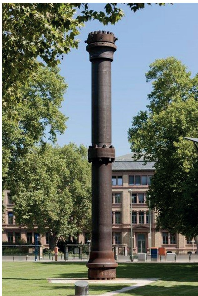
Figure 5. Photograph of an ammonia synthesis reactor from 1925, now exhibited in front of the BASF Gesellschaftshaus.
